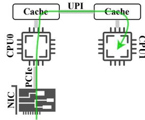
**Figure 2: The NIC can only transmit to its 'root' processor, and not directly to the processor core destined to process its data.**
